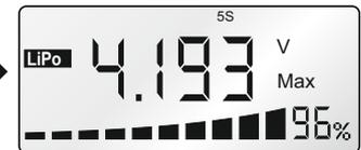
Shows the number of the cell with the highest voltage and the approximated remaining capacity.
