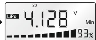
Shows the number of the cell with the lowest voltage and the approximated remaining capacity.
